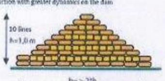
1 The sandbag dam should always be laid in a dense bond so that it is virtually impermeable. The use of film on the water side has also proved its worth.
