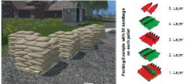
Packing Example with 50 sandbags on each pallet
